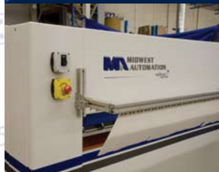
Infeed hold down roller kit prevents laminate curling.
