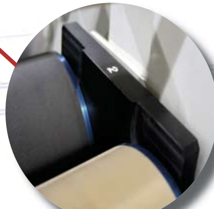
Spreading roller, ebonite dosing roller, and spring-loaded, Teflon end seal.
