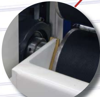
Spreading roller & glue dam with machined metering bar & brass end seal.
