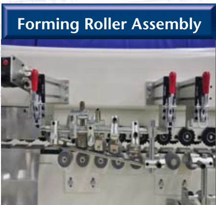
Quick-change forming roller assembly with over-center clamps to reduce set-up without special tools.
