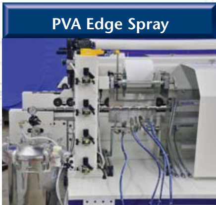
Optional PVA edge spray system for applying adhesive to the edge of core and laminate.
