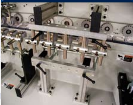
Side and underwrap compression roller assemblies with adjustable, spring-loaded silicone rollers.
