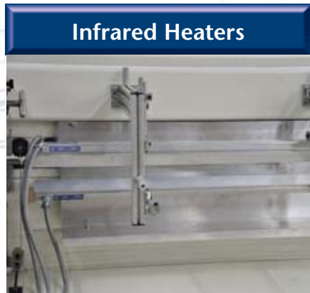
Top & bottom infrared heaters for heating laminate and drying adhesive.
