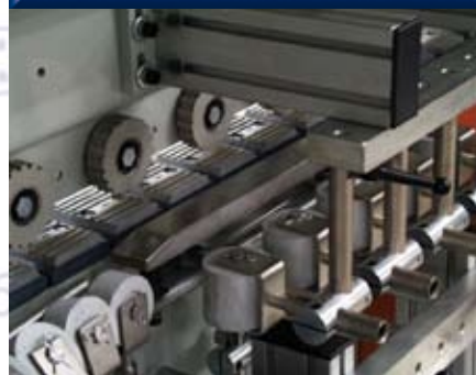
Compression shoe and rollers to facilitate PVA adhesive bonding.
