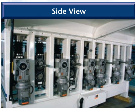
RP 4000/5000 with 6 driven upper rollers & pneumatic pressure control
