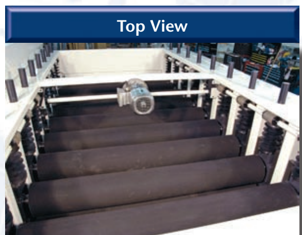
RP 4000/5000 with 10 rubber-coated, precision ground roller sections
