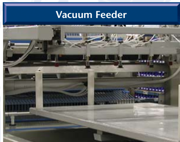
Automatic vacuum feeder for the HPL eliminates the need of an operator.
