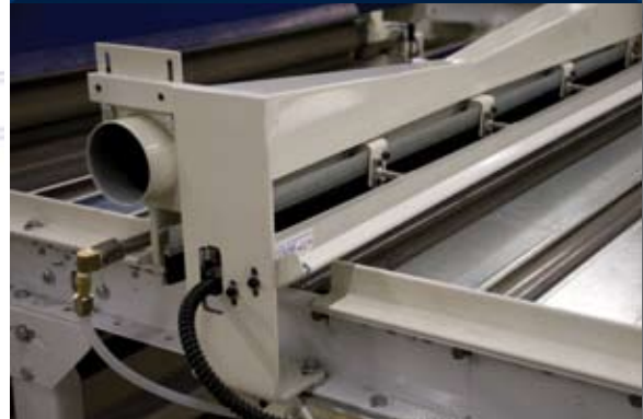
Special HPL cleaner with ionization unit, brush and vacuum pump.
