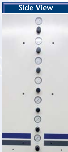
Pressure regulators for each spray gun
