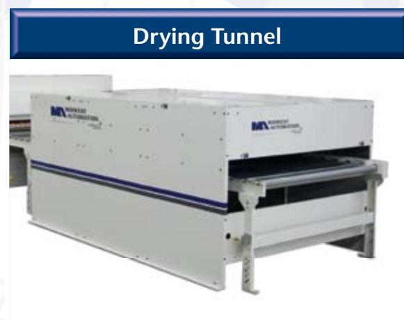
High efficient infrared drying tunnel with individually controlled heater banks.
