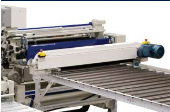
Special panel cleaner with cross belt design.
