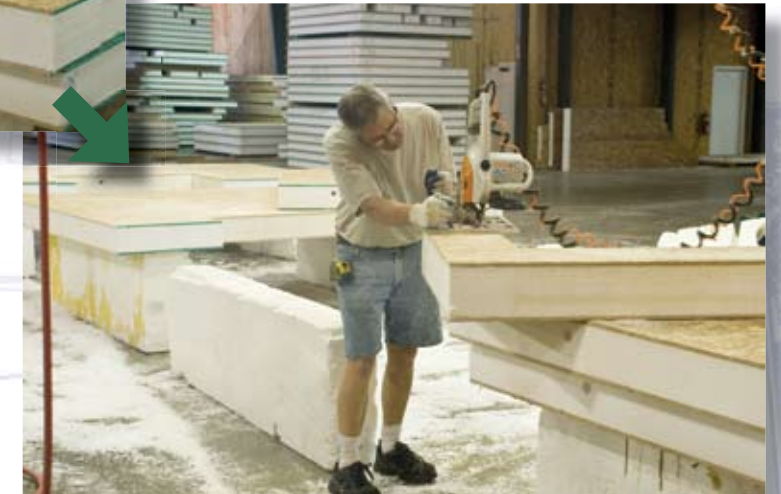
Operator using special chain saw for cutting a finished panel.
