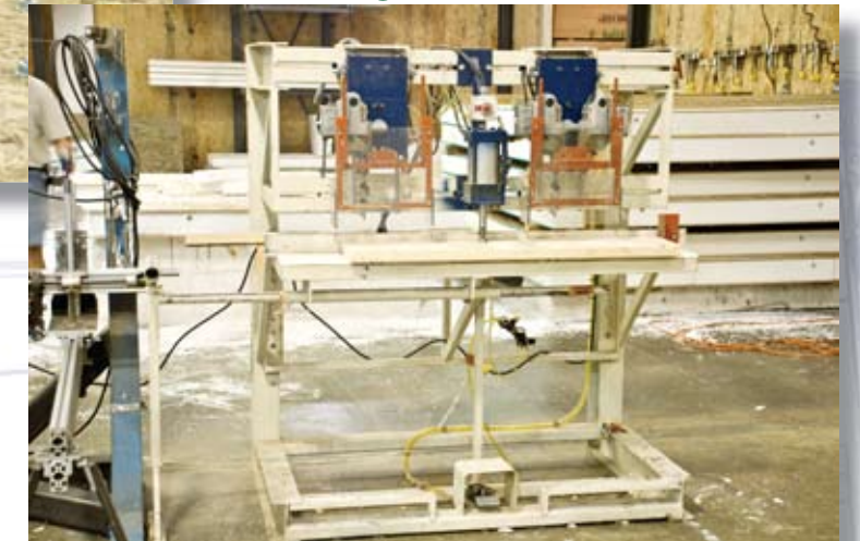
Multi-head press for drilling king post holes.
