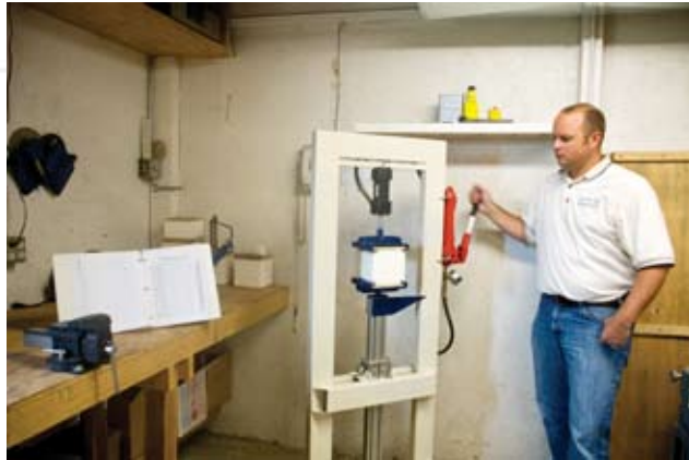
Pull test stand with hydraulic cylinder to measure internal bond strength of EPS and glue line.
